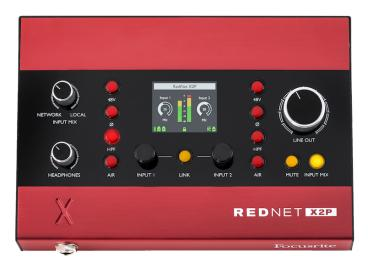
RedNet X2P incorporates two local Red Evolution mic/line/instrument preamp channels, plus two channels of premium D-A conversion for Dante audio-over-IP signals, to provide a stereo monitoring unit, featuring separate headphone and line outputs.
